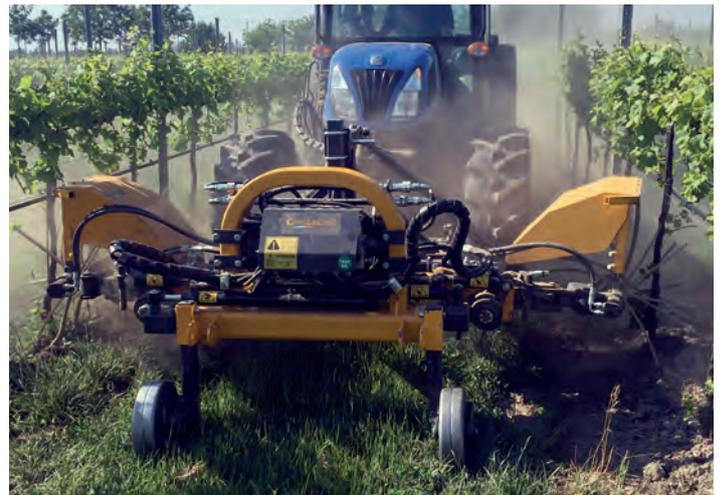
FAST con la testata spollonatrice - FAST with shoot removing head
