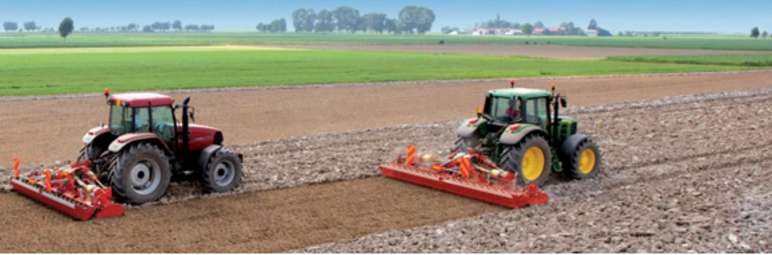
The Eternum power harrows are characterized by great ruggedness and reliability and are ideal for difficult working conditions. Thanks to their exceptionally long life, you will forget the year you bought them. Top strength frames, gears mounted on taper roller bearings, also available in patented model Rapident which allows a rapid replacement of the tines from the centre of the rotor.
